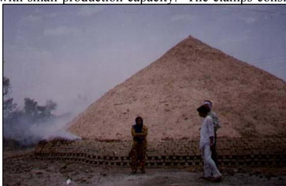
Since the whole stack of bricks is exposed to the atmosphere, heat loss from the surface is excessive. The production process is highly vulnerable to external weather conditions and the production period is usually limited to 120 days per annum. The firing cycle is offer duration of 21 to 28 days
